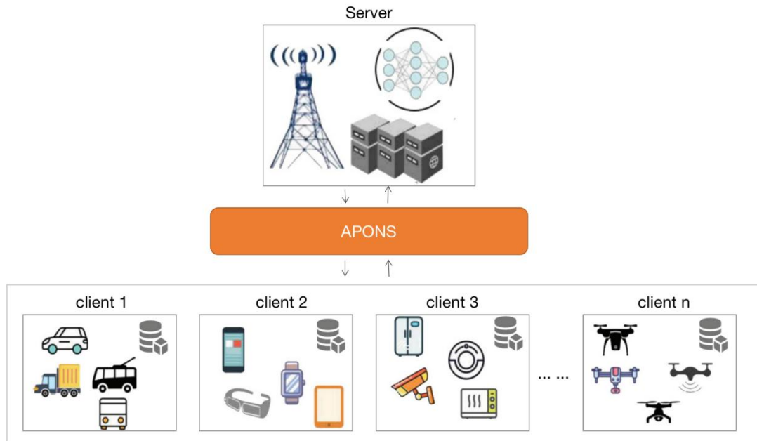
Figure 1: APONS training model on mobile edge computing enabled by 6G
